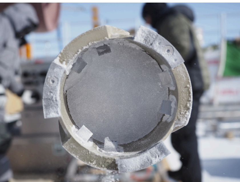
image: Ice core from 50 metres, taken with Eclipse drill. photo: Dr Joel Pedro/Australian Antarctic Division.
