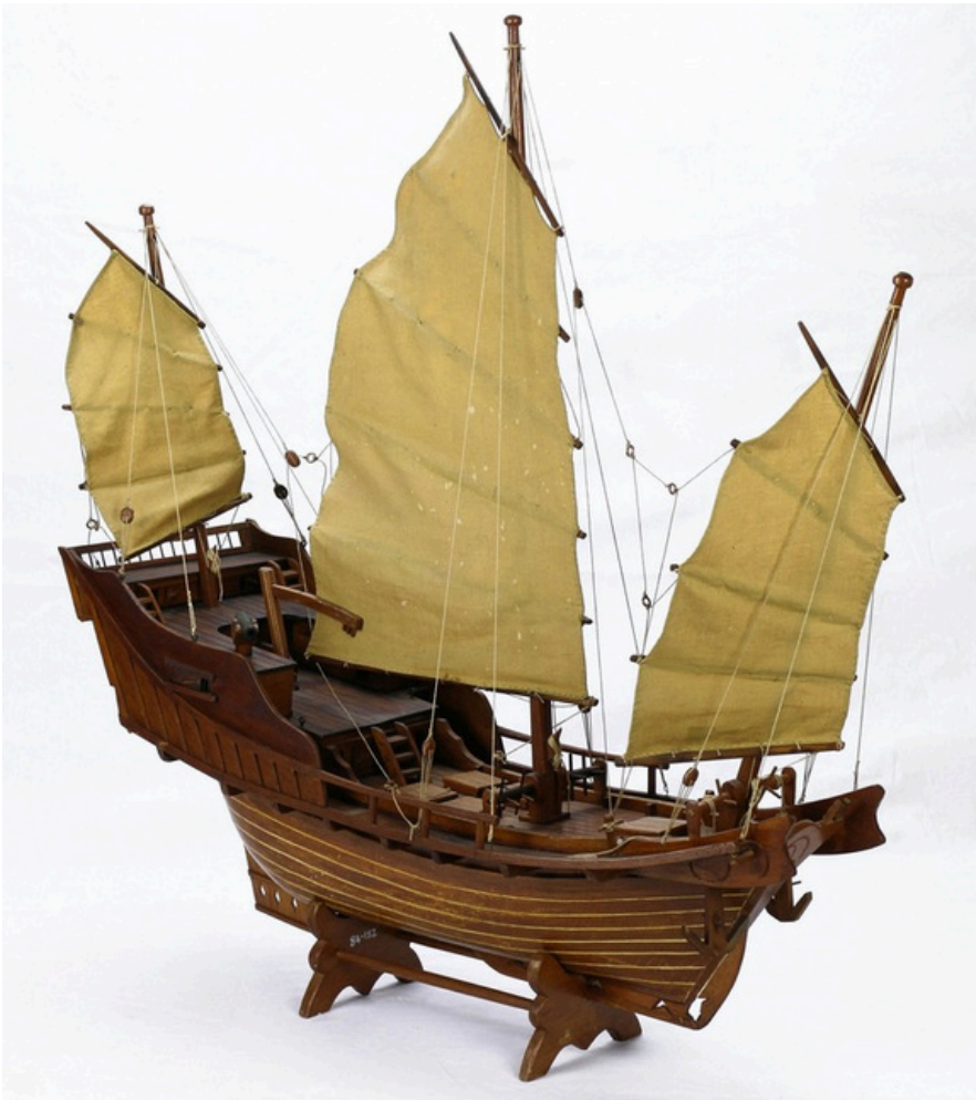
image: model of a Chinese ocean-going junk with a fully-rigged hull, late nineteenth-century (MMT collection A_1984-152)
