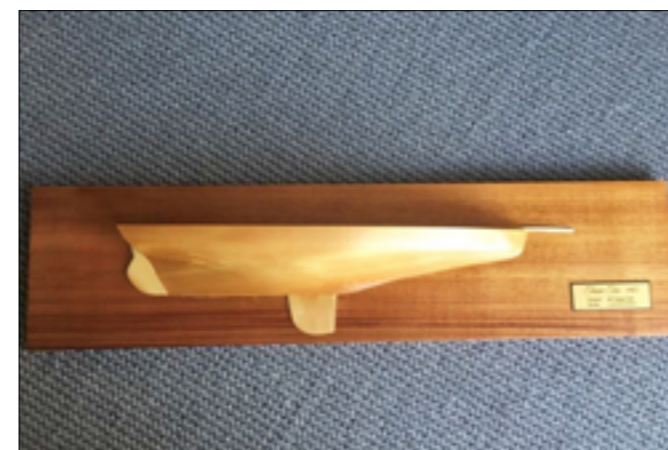
Figure 3. The Tassie Too half-model produced with a Computer Numerical Control (CNC) machine
