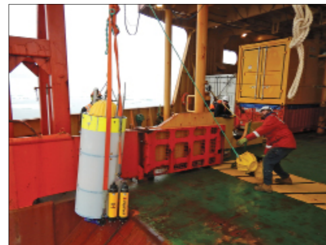
Acoustic mooring — After a year moored to the sea floor this acoustic mooring, being retrieved from the Southern Ocean, will contain more than 8000 hours of sound recordings.
