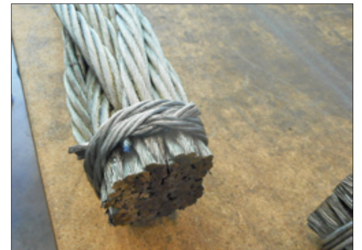
A graphic demonstration of the use of a Double Constrictor to hold a plaited steel cable for cutting. Raymond considers this his favourite knot, and it can be seen why.
