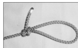
b-3 - To finish the knot and make it secure, make a Half Hitch around the Standing Part
