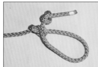
a-3 - Tie a Thumb Knot in the Working End to secure the knot
