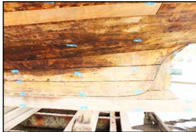
Figure 4-. Masking tape and dot targets on Coralyn
