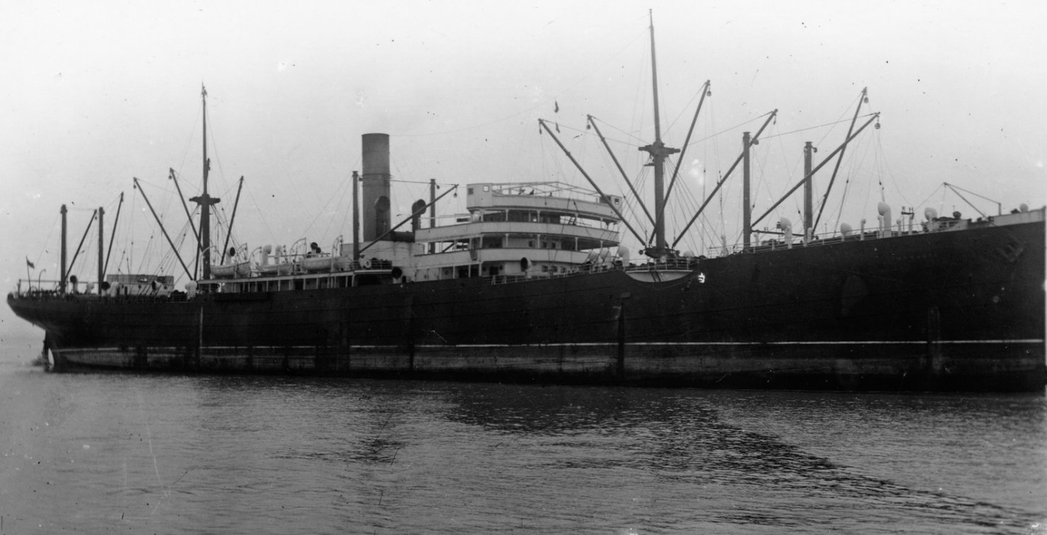
image: Tasmania in New Zealand Shipping Co. colours - the short well forward of the bridge was a common feature of German-Australian Line vessels. (Photographer unknown)
