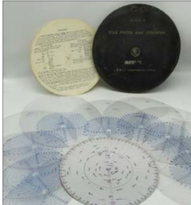
Star Finder and Identifier (US Navy Hydrographic Office - No.2102-D ) will be included in the 'Reimagining the Ocean' exhibition (p. 7). It consists of a round base plate and eight overlays with instruction page, all kept in a round plastic case, 245mm diameter.
