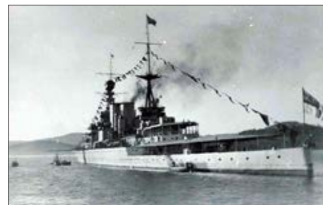
HMS Renown , a battlecruiser Gunnery included three twin-gunned turrets, anti-aircraft guns and two submerged torpedo tubes. It had armour with bulges to repel enemy torpedoes. Built: Fairfield Shipping & Engineering Co., Govan, Glasgow Launched 1916 Length overall: 794 feet 1.5 inches (242m) Beam 102 feet (31.1m) Draught (max.) 30 feet 3 inches (9.2 m). Displacement 26 500 tons Ref: Jane's Fighting Ships . Fred T Jane (ed.) Photo: MMT Collection P_ 2020-019
