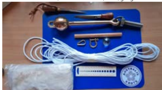
Tools and accessories for the Nuyina bell rope. From top left; fid, Swedish fid (both made by Mikko Snellman), bell clapper, dowel, brass thimble, brass shackle, glass knob, homemade 3.5mm hard laid cord, bleached shellac, ruler/gauge.
