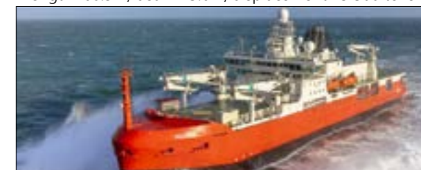
Icebreaker Nuyina length 160.3m, beam 25.6m, displacement 25 500 tons
